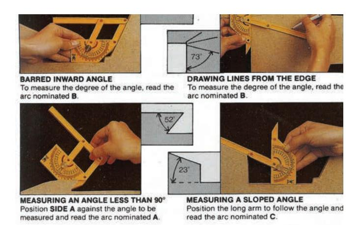
To rotate the protractor, position both arms over each other at the zero position. Tighten the top screw to secure your angle measurement.
