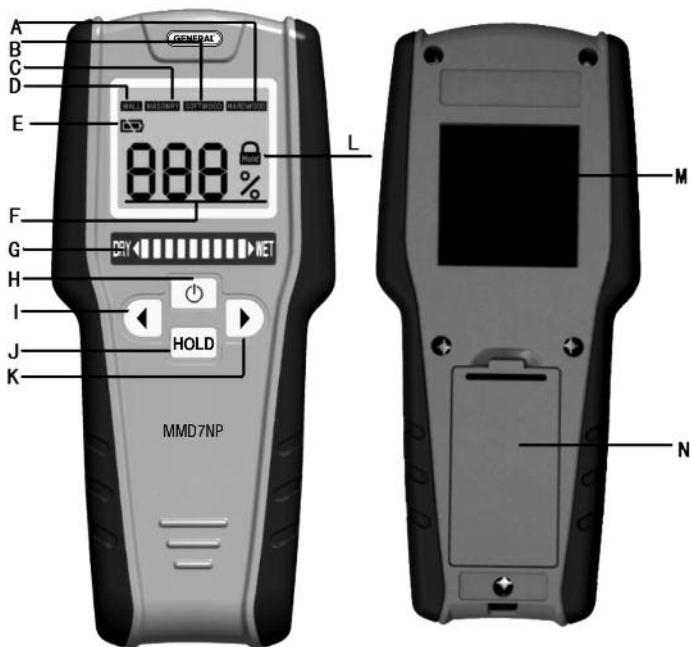
Fig. 1. The controls, indicators and physical features of the MMD7NP
