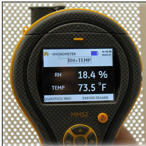
Figure 4: MMS2 as a Hygrometer
