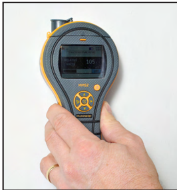
Figure 3: Taking Relative Moisture Readings
